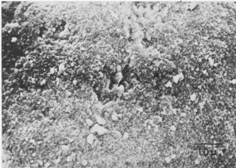
Figure 6. Scanning electron micrograph of the surface of charcoal granule with a coating thickness of about 1 μ (MC-5). The surface is still rough, while fine carbon particles are covered by the coating layer.
