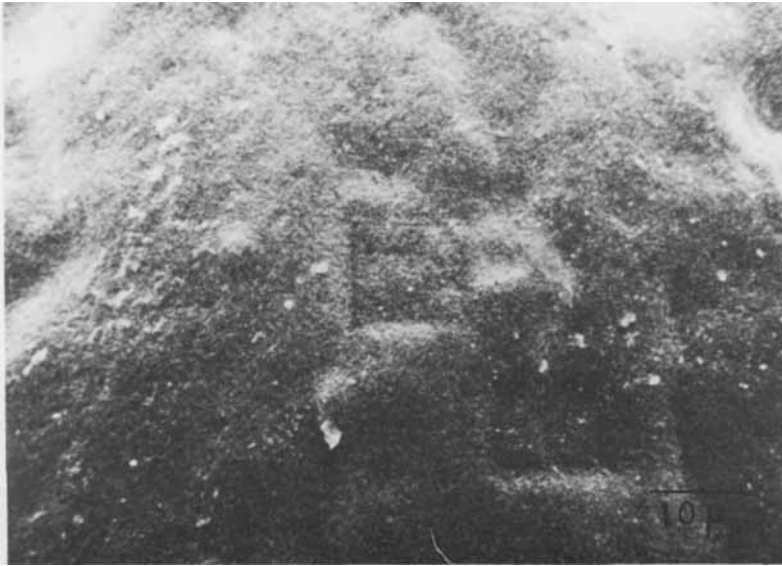
Figure 7. Scanning electron micrograph of the surface of charcoal granule with a coating thickness of about 3 \mu\text{m} (MC-6). The surface is completely smooth.
