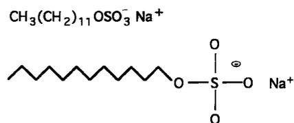
Figure 2.1 The chemical structure of sodium dodecyl sulfate.
