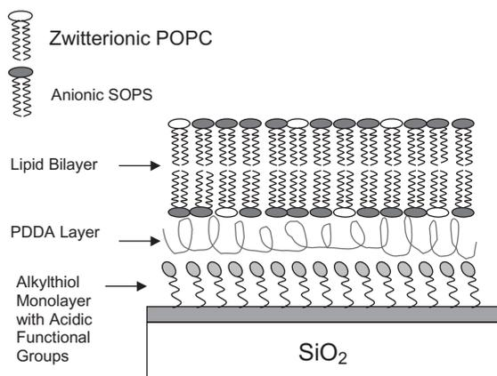
**Figure 2.7** Schematic representation of the model membrane system. The alkylthiol 11-mercaptoundecanoic acid (MUA) layer is self-assembled on a gold surface. The negatively charged head-groups of MUA
