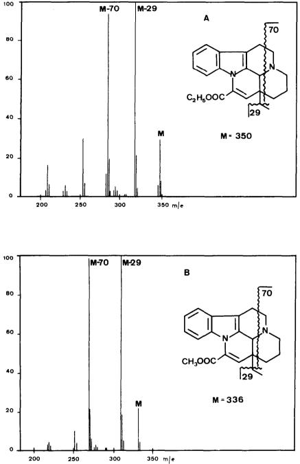
Fig. 1. Mass spectra of (A) vinpocetine and (B) internal standard.
