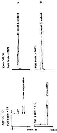
Fig. 2. SIM chromatograms of a plasma sample containing (A) 0.1 ng/ml and (B) 2 ng/ml vinpocetine; 10 ng/ml internal standard was added to each sample before extraction.
