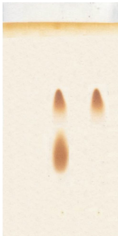
Figure 3. Photograph of the chromatogram showing resolution of racemic atenolol on L-tartaric acid impregnated plate. From left to right: spot 1, lower for ( R )-atenolol and upper for ( S )-atenolol; spot 2, pure ( S )-atenolol; mobile phase, CH 3 CN-CH 3 OH-CH 2 Cl 2 (3:3:4, v/v); run time, 15 min; solvent front, 8 cm; detection, iodine vapour. This figure is available in colour online at www.interscience.wiley.com/journal/bmc
