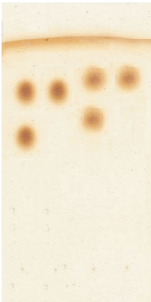
Figure 2. Photograph of the chromatogram showing resolution of racemic atenolol and propranolol on ( R )-mandelic acid impregnated plate. From left to right: spot 1, lower for ( R )-atenolol and upper for ( S )-atenolol; spot 2, pure ( S )-atenolol; spot 3, lower for ( R )-propranolol and upper for ( S )-propranolol; spot 4, pure ( S )-propranolol; mobile phase, CH 3 CN-CH 3 OH-HOAc (8:1:0.5, v/v); run time, 10 min; solvent front, 8 cm; detection, iodine vapour. This figure is available in colour online at www.interscience.wiley.com/journal/bmc
