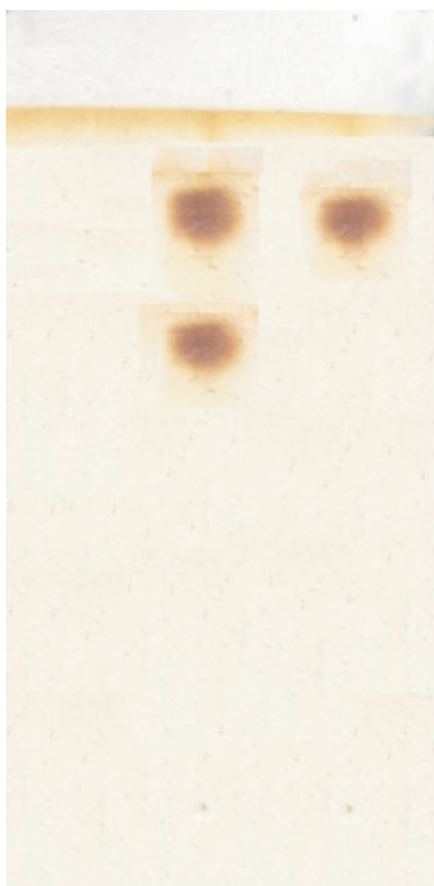
Figure 4. Photograph of the chromatogram showing resolution of racemic propranolol on L-tartaric acid impregnated plate. From left to right: spot 1, lower for ( R )-propranolol and upper for ( S )-propranolol; spot 2, pure ( S )-propranolol; mobile phase, CH 3 CN-CH 3 OH-HOAc (5:5:0.5, v/v); run time, 15 min; solvent front, 8 cm; detection, iodine vapour. This figure is available in colour online at www.interscience.wiley.com/journal/bmc
