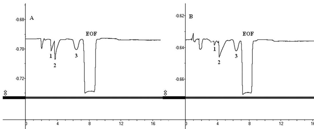
**Figure 2.** Typical electropherograms obtained when operated under the adopted conditions. (A) 150 µg/mL standard, (B) Teklo tablet. 1, Amiloride; 2, atenolol; and 3, internal standard (L-valine). Conditions: 150 mM acetic acid; voltage, 25 kV; temperature, 28°C; injection time, 25 s; and detector excitation signal, 100 V × 350 kHz.
