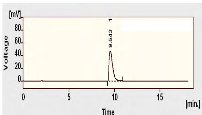
**Fig. 4.** Representative chromatogram of betahistine ( $320 \mu\text{g mL}^{-1}$ ) using YMC ODS column ( $250 \text{ mm} \times 4.6 \text{ mm}$ ,  $5 \mu\text{m}$ ) at a flow rate of  $2.0 \text{ mL/min}$ , detection at  $254 \text{ nm}$  with mobile phase  $\{60:40::\text{buffer solution (0.46\%, w/v, of NaH}_2\text{PO}_4, 0.27\%, \text{ w/v, of sodium dodecyl sulphate and 0.4\% hexylamine):acetonitrile}\}$ .
