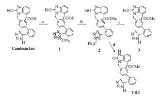
**Scheme 1.** Reagents and conditions: (a) TEA, trityl chloride,  $CH_2Cl_2$ ; (b) MeI,  $K_2CO_3$ , DMF, room temperature, 15 min; (c) HCl (1 N), DMF, 65–70 °C, 1 h; (d) HCl (1 N), DMF, 90 °C, 1.5 h. For [<sup>11</sup>C]methyl-candesartan: (b) [<sup>11</sup>C]MeI,  $K_2CO_3$ , Kryptofix, DMF, 65–70 °C, 3 min; (c) HCl (1 N), DMF, 65–70 °C, 2 min. For [<sup>11</sup>C]TH4: d) HCl (1 N), DMF, 90 °C, 2 min.
