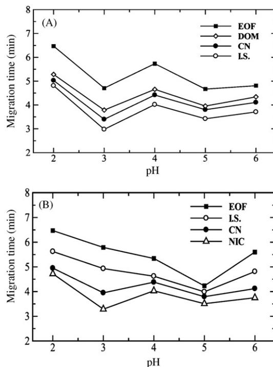
Fig. 3. Effect of pH on migration times of (A) CN/DOM/IS/EOF and (B) CN/NIC/IS/EOF. Buffers of glycine–HCl (pH 2.0) and acetate (pH 3.0–6.0) were used. The other conditions are the same as those in Fig. 2.
