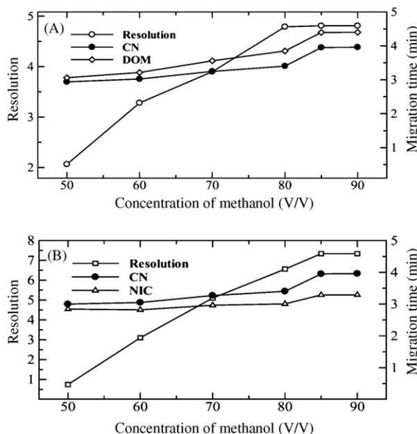
Fig. 2. Effect of methanol concentration on resolution and migration times. (A) CN (20 µg/ml) and DOM (15 µg/ml); (B) CN (25 µg/ml) and NIC (10 µg/ml). Running buffer, 10 mM acetate buffer (pH 3) containing various amounts of methanol; detection at 215 and 227 nm for (A) and (B), respectively; applied voltage, 20 kV; hydrodynamic injection, 25 mm for 30 s.
