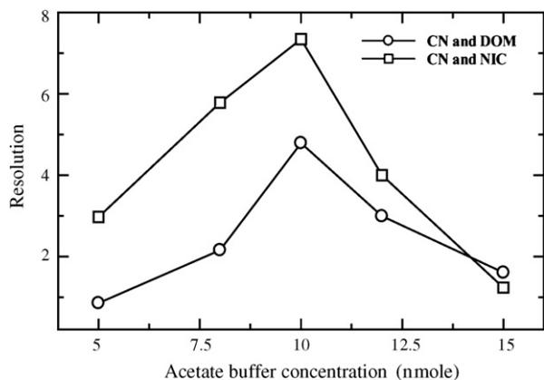
Fig. 4. Effect of acetate buffer (pH 3.0) concentration on the resolution of the separation of CN/DOM and CN/NIC. The other conditions are the same as those in Fig. 2.
