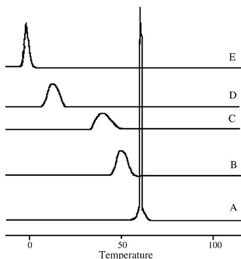
Fig. 1. DSC curves: (A) P 188/propylene glycol (100%/0%); (B) (99%/1%); (C) (98%/2%); (D) (97%/3%); (E) (0%/100%).
