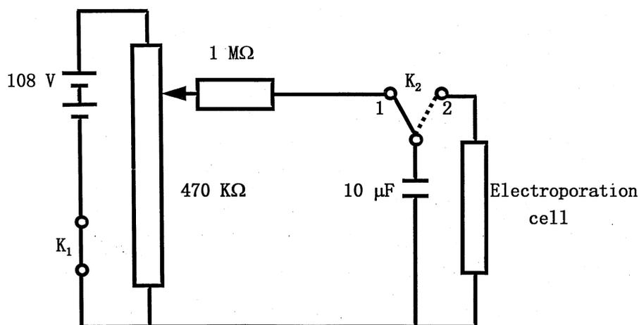
Fig. 1. Circuit diagram of the RC electric pulse generator.
