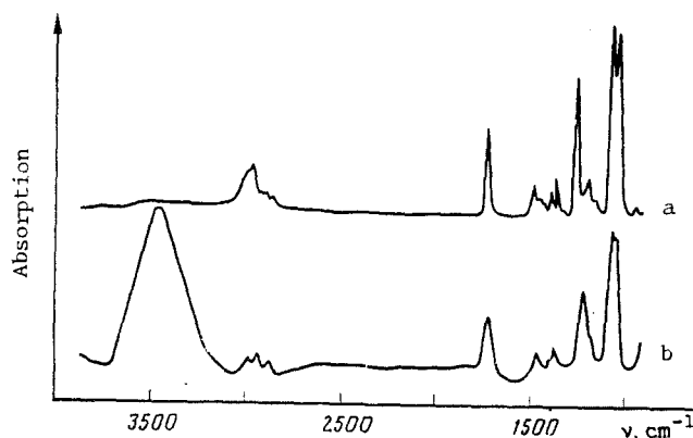
Fig. 1. IR spectrum of liquid DMP (a) and difference spectrum of its aqueous solution (b).
