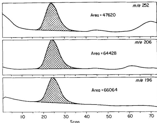
Figure 3. Selected ion monitoring data used to calculate the relative abundances and to identify GABA in a CSF sample.
