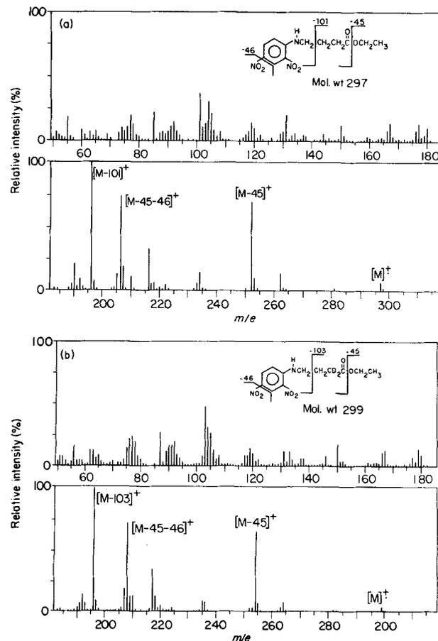
**Figure 2.** Mass spectra of the *N*-dinitrophenyl ethyl esters of (a) GABA; (b) [ $^2\text{H}_2$ ]GABA.
