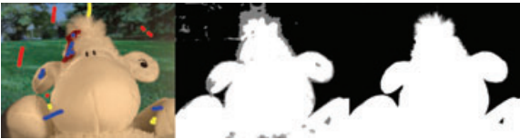
Figure 5: Use of our technique to interactively segment images by alpha matting. As the user scribbles over the image (left), a trimap is automatically updated. The resulting trimap and alpha matte computed from the set of scribbles on the left are shown on the center and right images.
