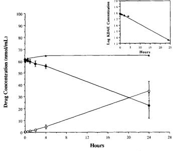
Figure 4—The enzymatic hydrolysis of KDAE upon incubation of human cadaver skin with ester solution at 32 °C. The inset is a log concentration versus time plot showing first-order metabolic degradation kinetics. Key: KEE (closed circle); KA (open circle); control, KDAE in buffer (open triangle).
