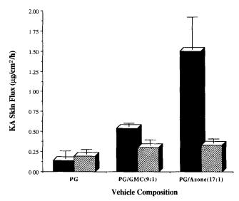
Figure 8—The skin flux of KA following application of KDAE (closed bar) and KEE (hatched bar) transdermal solution in the donor compartment. PG = propylene glycol; GMC = glyceryl monocapyrlate.
