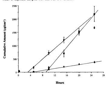
Figure 7—Representative permeation profiles for the diffusion of KA (closed circle), KEE (closed triangle), and KDAE (closed square) though human cadaver skin from PG/GMC (9:1) vehicle mixture at 32 °C.
