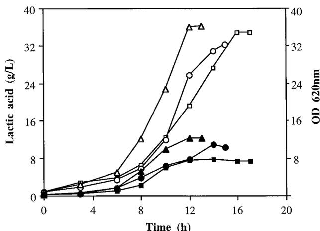
**Figure 2.** Lactic acid production (open symbols) and cell densities (closed symbols) during batch fermentation using free cells of *L. casei* in a culture medium of whey hydrolysate supplemented with (a) 2.5 g/L of yeast extract (○, ●), (b) 0.18 mM Mn<sup>2+</sup> (□, ■), and (c) 2.5 g/L of yeast extract and 0.18 mM Mn<sup>2+</sup> (Δ, ▲).
