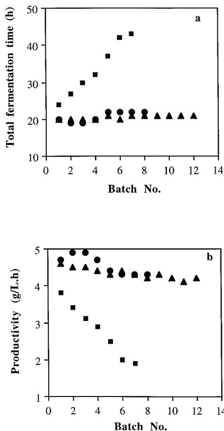
**Figure 5.** Time taken for fermentation (A) and reactor productivities (B) during repeated recycle batch fermentations in whey hydrolysate medium with *L. casei* adsorbed to Pora-bact A beads pretreated with 0% (■), 1% (●), and 2% (w/v) (▲) polyethyleneimine solution. To the medium were added 2.5 g/L yeast extract, 0.18 mM MnSO<sub>4</sub>, and glucose to a total reducing sugar concentration of 100 g/L.
