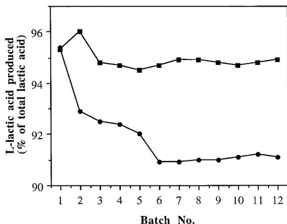
**Figure 7.** Yield of L-lactic acid in percent of total amount of lactic acid produced during repeated recycle batch fermentation with immobilized *L. casei* in the medium supplemented with 1 g/L (■) and 2.5 g/L (●) of yeast extract, respectively.
