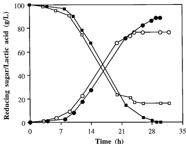
**Figure 3.** Batch lactic acid fermentation with free *L. casei* cells in whey hydrolysate medium supplemented with 2.5 g/L of yeast extract, 0.18 mM  $MnSO_4$ , and lactose (closed symbols) or glucose (open symbols) making the total reducing sugar concentration 100 g/L. The sugar consumption is shown as square symbols, and lactic acid production as circles.
