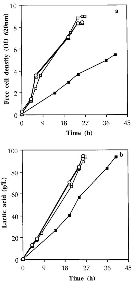
**Figure 8.** Profiles of free cell density (A) and lactic acid formation (B) during repeated recycle batch fermentations in a bioreactor, which was inoculated by circulating the culture broth from an actively running recycle batch reactor. Fermentation cycles: first (■), second (□), third (●), and fourth (○). Experimental details given in the text.
