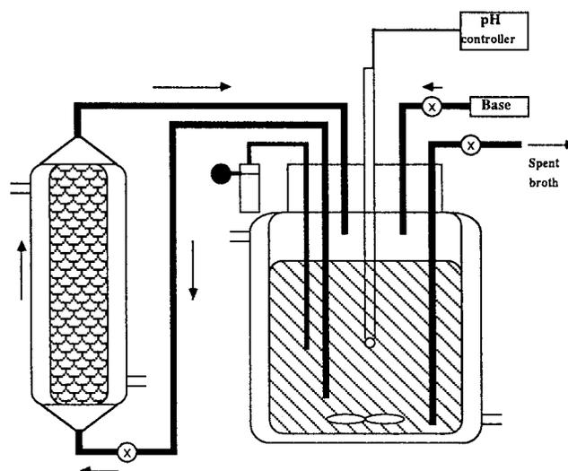
**Figure 1.** Schematic diagram of the experimental set-up used for lactic acid fermentation by immobilized *Lactobacillus casei* cells. The details are provided in the text. The arrows indicate the circulation of culture medium in the reactor system.
