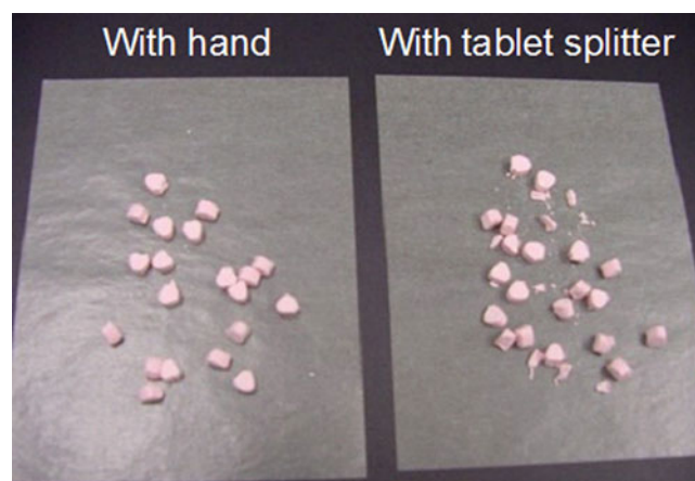
Fig. 2. Marketed levothyroxine tablets (L-3) cut with hand and tablet splitter. Tablet splitter produced more fragments for all the tablets (only figure for L-3 is shown here)
