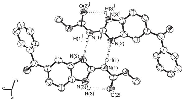
**Figure 3.** MBZ dimer projected onto the plane (123) showing the strong intermolecular N(1)–H(1)···N(2) hydrogen bond connecting the molecules, likewise the moderate intramolecular N(3)–H(3)···O(2) interaction can be evidenced. Double dotted lines illustrate the hydrogen bonds. The H-atoms involved in the hydrogen bonds are shown as spheres of arbitrary radii. Symmetry code: (i)  $-x; 1-y; -z$ .
