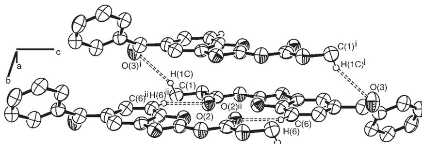
**Figure 4.** Weak nonclassical hydrogen bonds contributing to MBZ crystal packing along the directions [123] (symmetry operator: (i)  $1-x; -y; -z$ ) and  $[2, -1, -3]$  (symmetry operator: (ii)  $2-x; -y; -z$ ). Double dotted lines represent the intermolecular hydrogen bonds. The H-atoms involved in the hydrogen bonds are shown as spheres of arbitrary radii.
