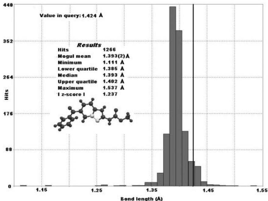
**Figure 6.** Histogram comparing the N(2)–C(4) bond length of MBZ with the equivalent distances of resembled compounds found in CSD.
