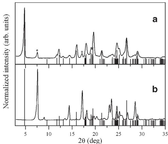
**Figure 7.** Comparison among the X-ray powder peak positions from MBZ single crystal structure (vertical bars) and diffractograms (full line) of a form C rich mixture containing the mebendazole polymorphs A and C (a) and raw mebendazole polymorph A (b). The asterisks represent the most intense Bragg reflections of phase A that appear in the form C rich mixture.
