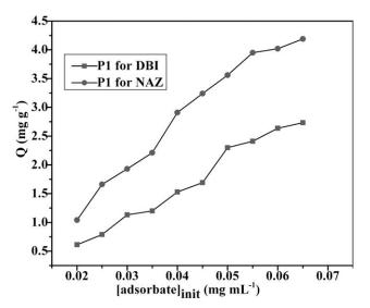
**Figure 3** Binding isotherms of P1 for NAZ and DBI [adsorbate]<sub>init</sub> is the initial concentration of NAZ or DBI.
