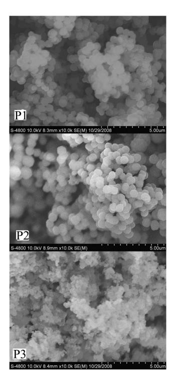
**Figure 2** Scanning electron micrographs of naphalazoline-imprinted microspheres using dichloromethane (P1), acetonitrile (P2) and Methanol (P3) as porogenic solvents.
