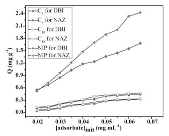
Figure 4 Binding isotherms of NIP,  $C_8$  and  $C_{18}$  for NAZ and DBI [adsorbate]<sub>init</sub> is the initial concentration of NAZ or DBI.
