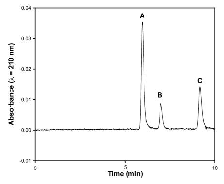
Fig. 1. Electropherogram of a sample containing the three components: A, NAPH; B, PHE and C, DIP, using a buffer phosphate solution of 0.063 mol  $1^{-1}$ , pH 3.72 and a voltage of 17.7 kV.
