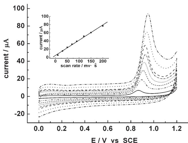
Fig. 4. Influences of scan rate on the electrochemical oxidation peak current of  $5 \times 10^{-6}$  M ofloxacin at MWNTs-CR/GCE in 0.1 M PBS (pH 6.0): 20, 40, 60, 80, 100, 120, 150, 200 mV/s. Inset: plot of the peak current vs. scan rate.
