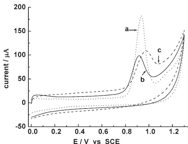
Fig. 3. Cyclic voltammograms of  $2 \times 10^{-5}$  M ofloxacin at MWNTs-CR/GCE (curve a), MWNTs - DHP/GCE (curve b) and MWNTs-Nafion/GCE (curve c) in 0.1 M PBS (pH 6.0). Scan rate: 100 mV/s.
