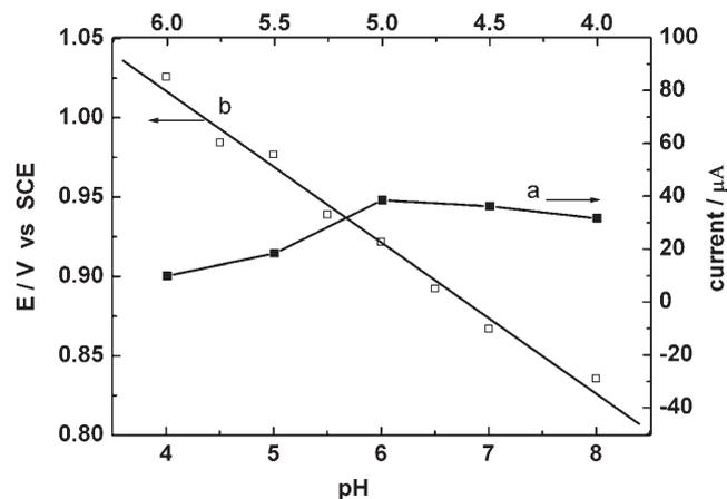
Fig. 5. Dependence of pH on peak current (a) and peak potential (b) of  $5 \times 10^{-6}$  M ofloxacin at MWNTs-CR/GCE in 0.1 M PBS. Scan rate: 100 mV/s.
