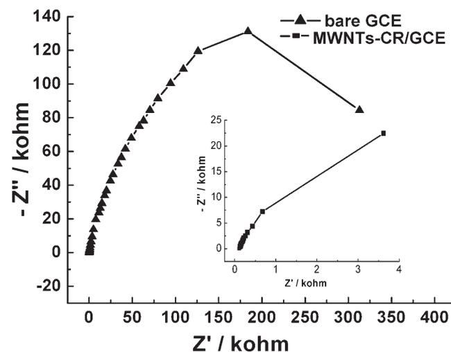
Fig. 1. The impedance responses of  $5 \times 10^{-6}$  M ofloxacin at the MWNTs-CR/GCE (■) and bare GCE (▲). Frequency range used: 100 kHz to 0.1 Hz with single amplitude of 5 mV rms at five steps per decade.
