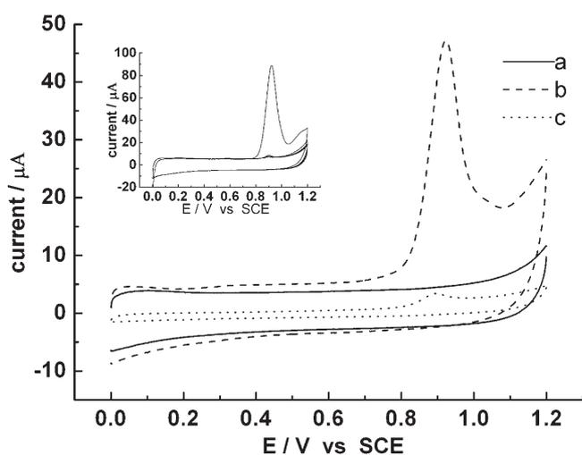
Fig. 2. Cyclic voltammograms of MWNTs-CR/GCE in the absence (curve a) and presence of  $5 \times 10^{-6}$  M ofloxacin at bare GCE (curve c) and MWNTs-CR/GCE (curve b) in 0.1 M PBS (pH 6.0). Scan rate: 100 mV/s. Inset: successive cyclic voltammograms of  $1 \times 10^{-5}$  M ofloxacin in 0.1 M PBS (pH 6.0) at MWNTs-CR/GCE. Scan rate: 100 mV/s.
