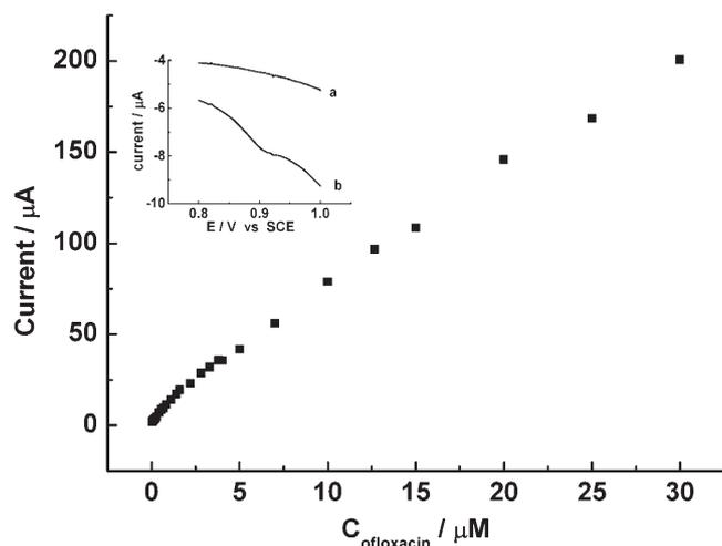
Fig. 6. Plot of the peak current vs. the concentration of ofloxacin. Inset: the voltammograms of MWNTs-CR/GCE in the absence (curve a) and presence of 9 nM ofloxacin (curve b). Scan rate: 100 mV/s.
