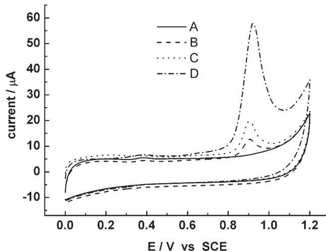
Fig. 7. Cyclic voltammograms of MWNTs-CR/GCE in urine assays without ofloxacin (curve A) and sample A (curve B), sample B (curve C) and sample C (curve D) with expected ofloxacin. Scan rate: 100 mV/s.
