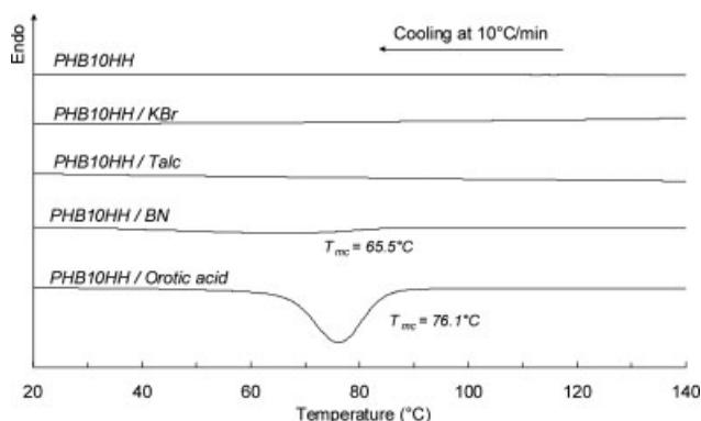
**Figure 3** DSC curves recorded during nonisothermal melt crystallization at 10°C/min of P(HB-co-10%HH) (PHB10HH) and their blends with potassium bromide (KBr, 1 wt %), talc (1 wt %), boron nitride (BN, 1 wt %) and orotic acid (1 wt %).
