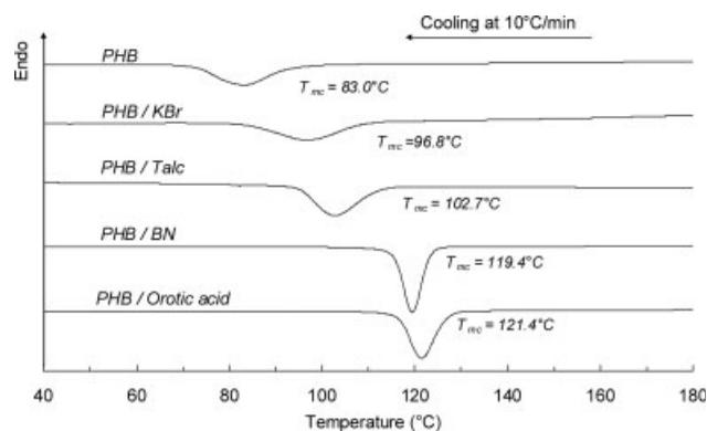
**Figure 2** DSC curves recorded during nonisothermal melt crystallization at 10°C/min of PHB and their blends with potassium bromide (KBr, 1 wt %), talc (1 wt %), boron nitride (BN, 1 wt %), and orotic acid (1 wt %).
