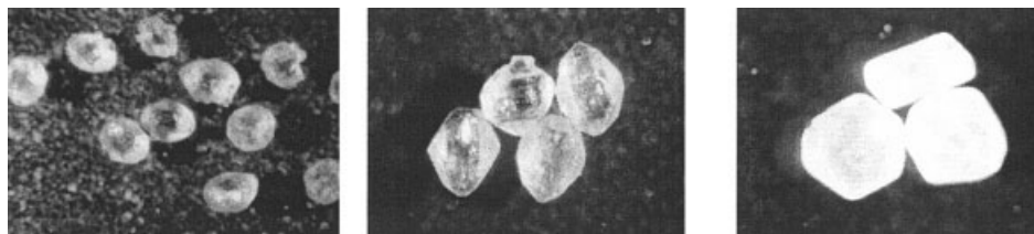
Figure 2. Paracetamol crystals (a) from aqueous solution with a cooling rate of 0.5°C/min, (b) seed crystals, and (c) product crystals from the (3 + 92.15 + 4.85) mixture.
