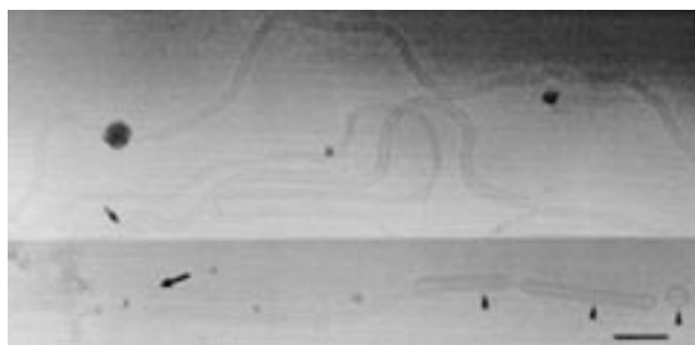
Figure 3. Macrocyclic phosphocholine A vesicle suspension observed in the frozen hydrated state. Mainly unilamellar tubules several micron long and around 300 Å in diameter are observed. As the images were not taken under low dose conditions the bilayer appears as a single line. A few unilamellar vesicles are observed (small arrow). Sometimes several microtubules are connected to each other through a narrow tether, the microtubule is fused with a spherical vesicle (large arrow) or includes a second vesicle (arrow heads). Scale bar: 200 nm.
