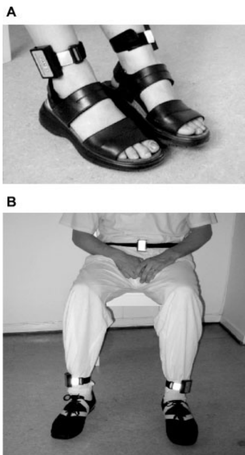
FIG. 1. Three-channel actometry: Two of the authors presenting the actometric monitors worn by the study subjects. Attachment around ankles ( A ; monitor on the lateral side) and waist ( B ; monitor on the anterior midline).
