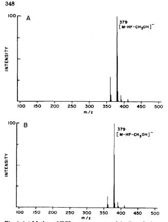
Fig. 4. (a) Methane NICI mass spectrum of the first eluting rimantadine diastereomer (labelled A in Fig. 2). (b) Methane NICI mass spectrum of the second eluting rimantadine diastereomer (labelled B in Fig. 2).
