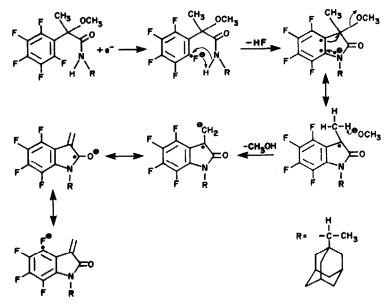
Fig. 5. Mechanism of formation of m/z 379.
