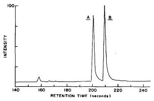
Fig. 2. Total ion current chromatogram from derivatized rimantadine. The mass spectrometer was set to scan from m/z 100 to m/z 500 with the GC temperature programmed in a manner similar to that described in the experimental section.
