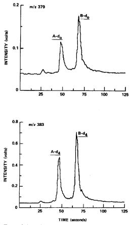
Fig. 6. Selected ion current profiles from a 72-h post-dose plasma sample from a subject given 200 mg of rimantadine. The 1.0-ml sample was fortified with 100 ng of tetradeuterated rimantadine. The chromatograms of the rimantadine- $d_0$  diastereomers are labelled A- $d_0$  and B- $d_0$  and those from the rimantadine- $d_4$  diastereomers are labelled A- $d_4$  and B- $d_4$ . (The times shown are relative to the beginning of data acquisition.)
