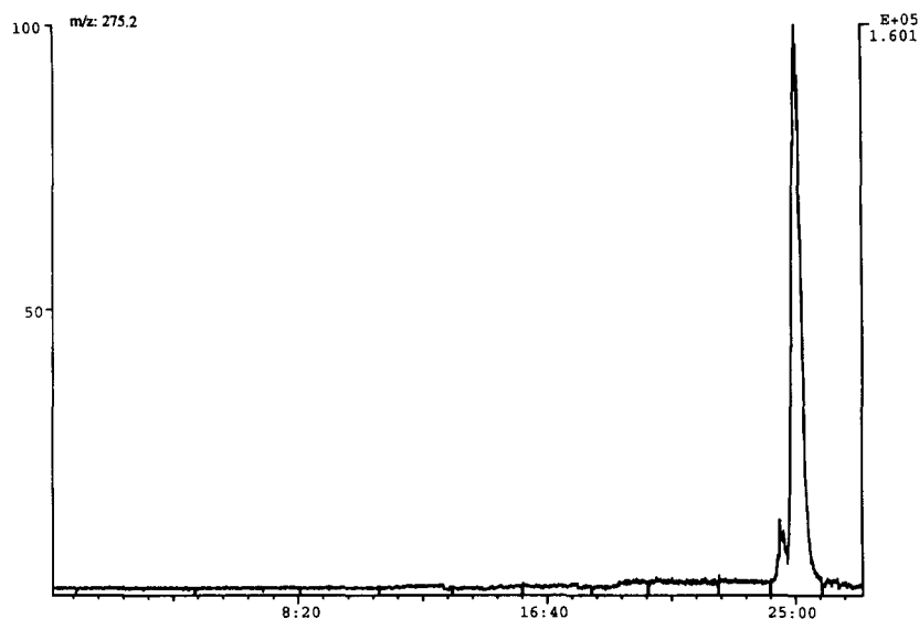
Fig. 6. Mass electropherogram obtained after chiral separation of a 1:20 mixture of ( R )- and ( S )-ropivacaine. The injected amount of ( S )-ropivacaine was 230 pg.
