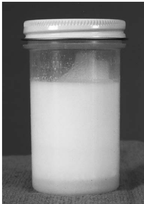
Fig. 2 Visible layering of sevelamer resin in human breast milk after as little as 10 min of pretreatment at 3^{\circ}\text{C}
