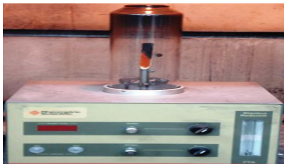
Fig. 2. Limiting oxygen index (LOI) chamber.
