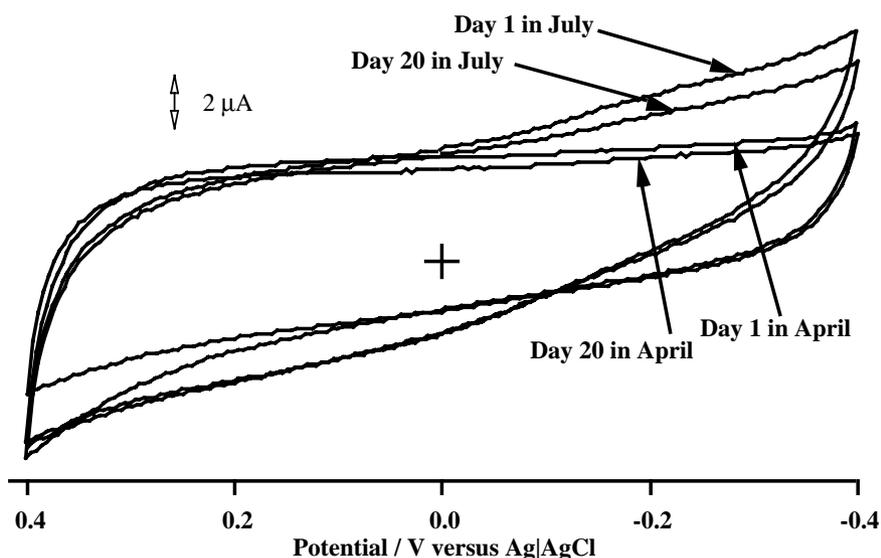
Fig. 4. Comparison of cyclic voltammetric response at thioctic acid SAM-coated gold electrodes in 0.1 M  $\text{KNO}_3$  in Day 1 and Day 20 over a 3-month period; scan rate =  $500 \text{ mV s}^{-1}$ .
