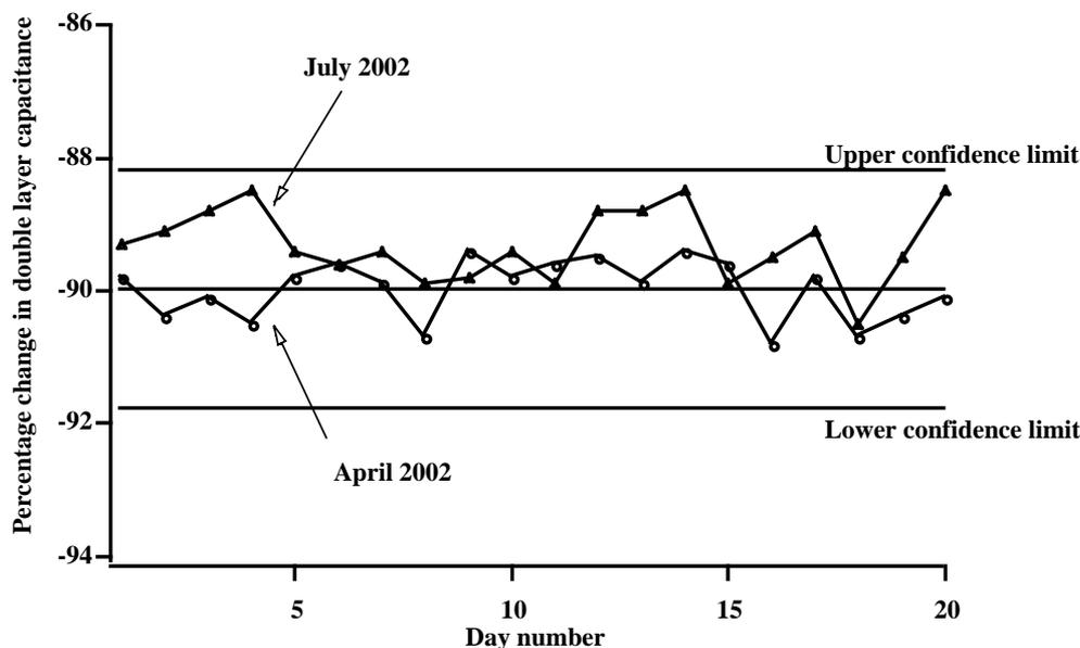
Fig. 5. A control chart with 99.7% confidence limits showing the percentage change in double layer capacitance of two electrodes over a 20-day period.
