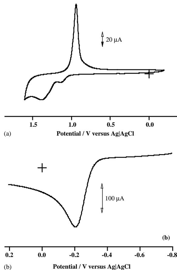
Fig. 1. (a) Cyclic voltammogram of 0.5 M  $\text{H}_2\text{SO}_4$  at a clean gold electrode; scan rate =  $500 \text{ mV s}^{-1}$ . (b) Linear scan voltammogram of 5.0 mM  $\text{Fe}(\text{CN})_6^{4-}$  in 1.0 M of  $\text{KNO}_3$  as supporting electrolyte; scan rate =  $50 \text{ mV s}^{-1}$ . In each voltammogram, the cross represents zero current position.
