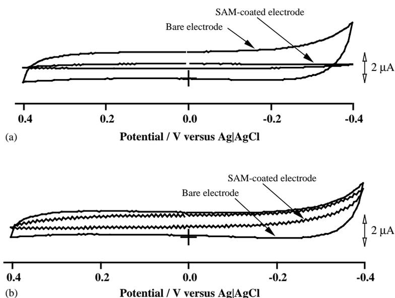
Fig. 2. Comparison of cyclic voltammograms of 0.1 M  $\text{KNO}_3$  at a bare gold electrode and a thioctic acid SAM-coated gold electrode using: (a) a direct application method and (b) an immersion method; scan rate =  $500 \text{ mV s}^{-1}$ .
