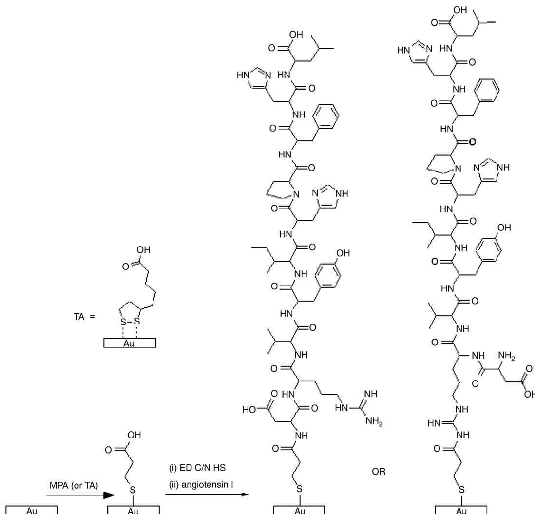
Scheme 1. General experimental conditions for the fabrication of MPA–angiotensin I and TA–angiotensin I modified gold electrodes. Electrodes are modified in 10 mM MPA/TA solution overnight followed by activation of the carboxyl groups using EDC/NHS to allow for the attachment of angiotensin I. Angiotensin I can attach to MPA/TA through the amino end of the Arg or Asp residue.
