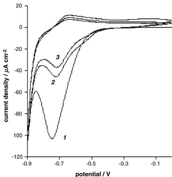
Fig. 4. Cyclic voltammogram in 50 mM ammonium acetate buffer (pH 7.0) containing 50 mM NaCl showing the region of desorption of TA modified electrodes. Scan rate: 0.1 V.
