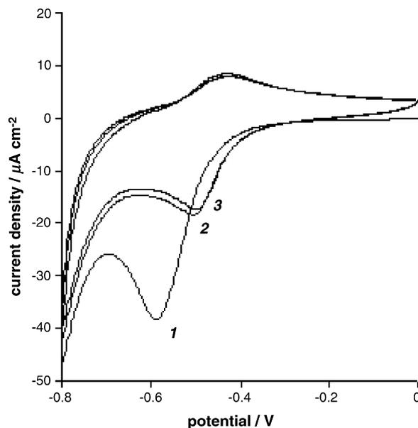
Fig. 2. Cyclic voltammogram in 50 mM ammonium acetate buffer (pH 7) containing 50 mM NaCl showing the region of desorption of MPA modified electrodes. Scan rate:  $0.1 \text{ V s}^{-1}$ .
