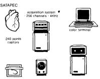
\* SATAPEC: 256-channel simultaneous acquisition system - automatic processing of cardiac electric potentials.
