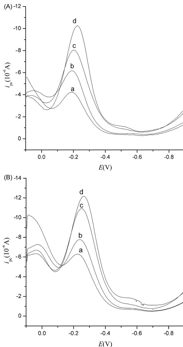
**Fig. 5.** Differential-pulse adsorptive stripping voltammograms (A) and square-wave adsorptive stripping voltammograms (B) in Britton–Robinson buffer at pH 7.0 after 30 s of accumulation for  $2.0 \times 10^{-7}$  mol/L (a),  $4.0 \times 10^{-7}$  mol/L (b),  $6.0 \times 10^{-7}$  mol/L (c) and  $8.0 \times 10^{-7}$  mol/L (d) valsartan. Other conditions as in Fig. 4.
