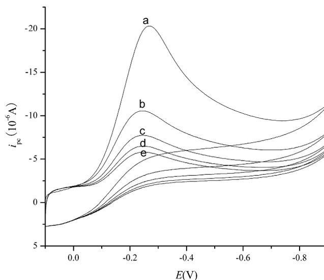
**Fig. 1.** Repetitive cyclic voltammograms obtained from a  $2.0 \times 10^{-6} \text{ mol/L}$  solution of valsartan after accumulation 30 s in Britton–Robinson buffer at pH 7.0. Scan rate:  $100 \text{ mV/s}$ . Curve “a”, first scan; curve “b”, second scan; curve “c”, third scan; curve “d”, fourth scan and curve “e”, fifth scan.
