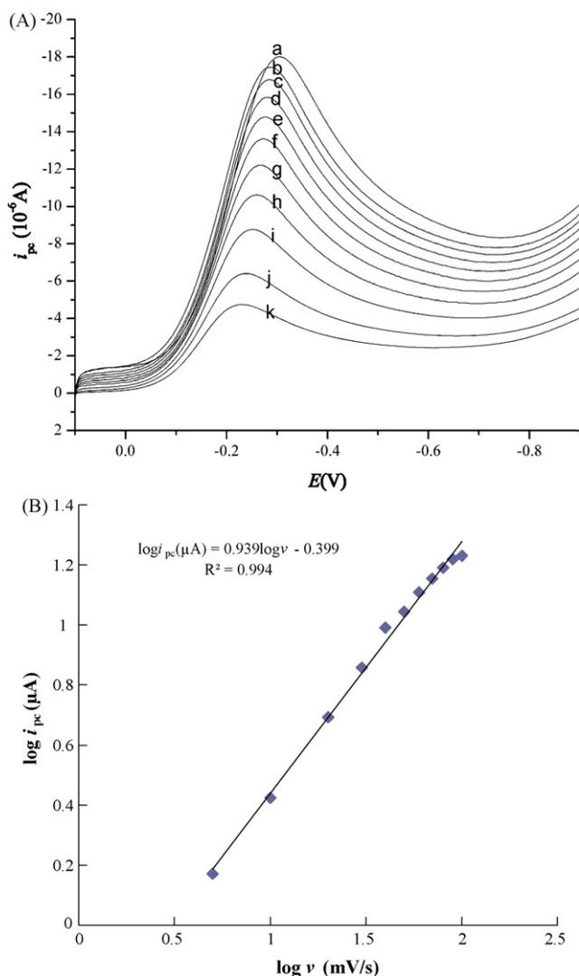
**Fig. 2.** Linear sweep voltammograms (A) obtained from a  $2.0 \times 10^{-6}$  mol/L solution of valsartan after accumulation 30 s in Britton–Robinson buffer at pH 7.0. Scan rate: curve “a”, 100 mV/s; curve “b”, 90 mV/s; curve “c”, 80 mV/s; curve “d”, 70 mV/s; curve “e”, 60 mV/s; curve “f”, 50 mV/s; curve “g”, 40 mV/s; curve “h”, 30 mV/s; curve “i”, 20 mV/s; curve “j”, 10 mV/s; curve “k”, 5 mV/s. (B) Plot of  $\log i_{pc}$  vs.  $\log \nu$ .
