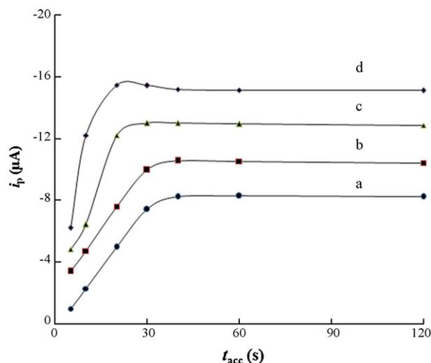
**Fig. 3.** Effect of accumulation time on the stripping cathodic peak current for  $6.0 \times 10^{-7}$  mol/L (a),  $8.0 \times 10^{-7}$  mol/L (b),  $1.0 \times 10^{-6}$  mol/L (c) and  $1.2 \times 10^{-6}$  mol/L (d) valsartan. Other conditions as in Fig. 2.
