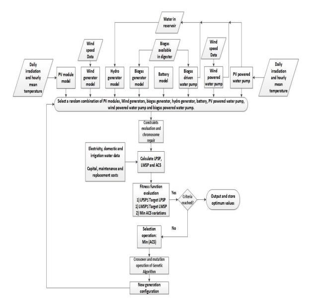
Figure 4. Flowchart for optimal sizing of SIRES using GA.
