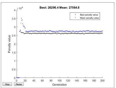
Figure 7. Variations of ACS during GA optimization process for diesel generator.
